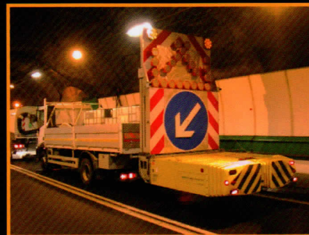
Truck with crash absorber (TMA) and brightly panel (fig. 401).
