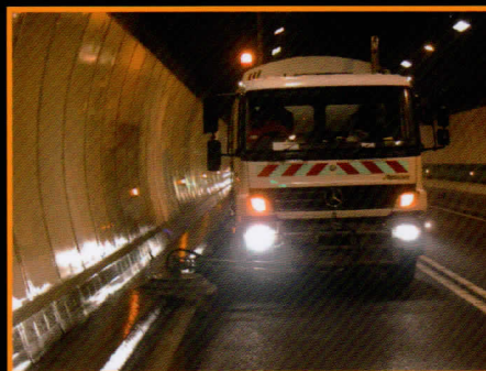
18.000 lt/min. liquid aspirator road sweeper with a third brush to clean sidewalk.
