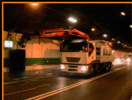
12.000 liters tank truck for the rotolavaggio and rinsing.
