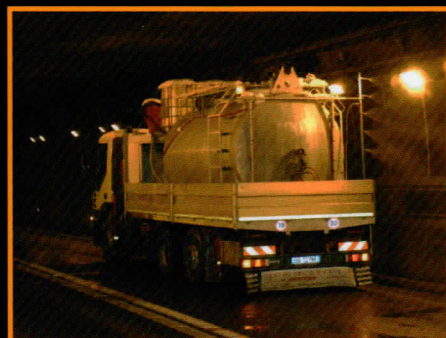
10.000 liters tank truck for detergent spraying.
